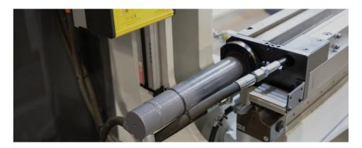
The crowning-construction balances the elastic deformation of the bedplate and the crosshead of the Press. Calculation an automatic setup occurs by the CNC. Automatic calculation and positioning of the crowning depend on the pressure surface and the bending position.
