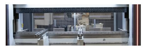
Exclusive bottom tool clamping system allows quick removal of tools. It has very precise holding and automatic tool centering.
