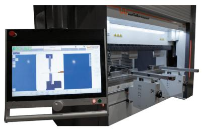
All Weinbrenner Press Brakes can be equipped with advanced CNC controllers. Highly effective CNC controllers optimize the machine cycle and minimize set-up time. These controllers make using press brakes easier, more efficient and more functional.
