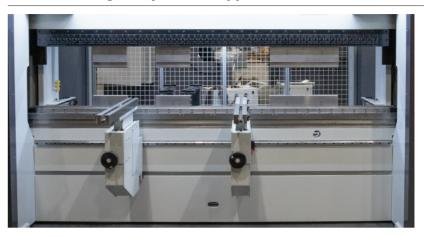
Weinbrenner Press Brakes offers newly designed Manuel Height Adjustable Support Arms. The mechanism equipped with a reducer and rack-pinion to adjust height easily.
