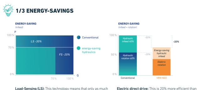
**Load-Sensing (LS):** This technology means that only as much hydraulic pressure (p) is built up for the position of the rollers as is required in actual operation. This leads to impressive energy savings of 30% with load sensing, particularly at partial load.
